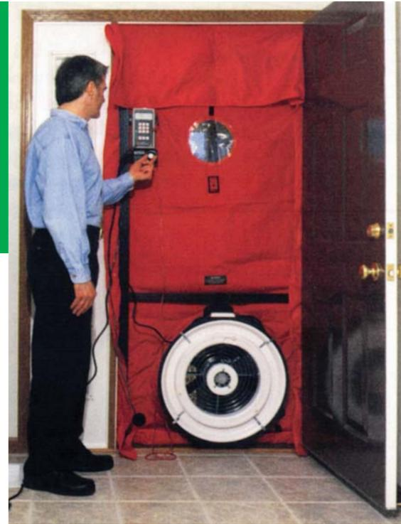
*A trained technician can easily fit pressure test equipment to most types of door installed in new dwellings*
